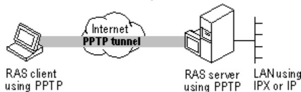
In the second example, the same functionality is achieved by calling an ISP instead of being directly connected to the Internet. The client first makes a call to the ISP. After that connection is established, the client makes another call to the RAS sever that establishes the PPTP tunnel.
